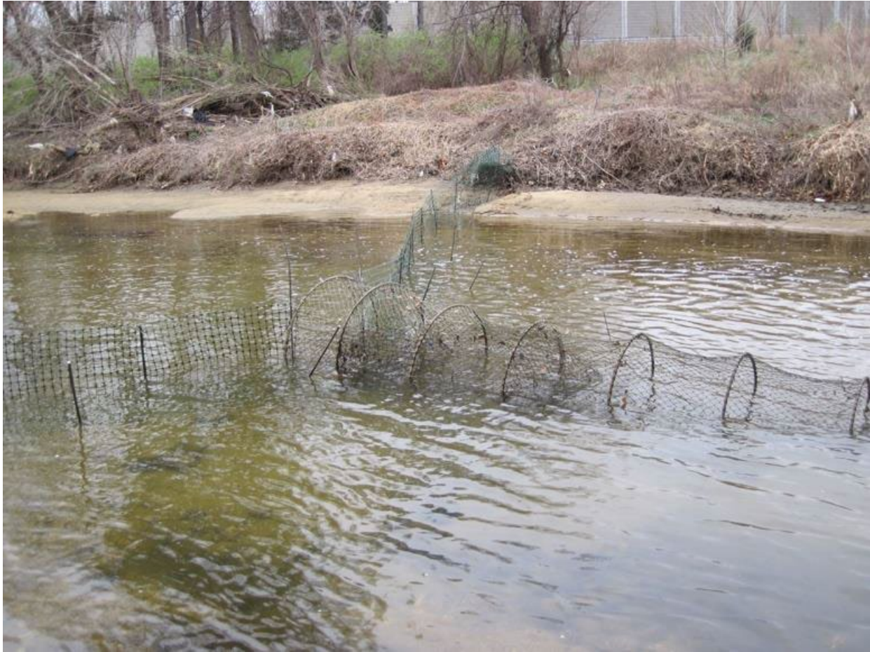
Figure 2. Hoop net deployed in new location in Cameron Run. The hedging is angled downstream in order to funnel up-migrating herring into the opening of the net.
