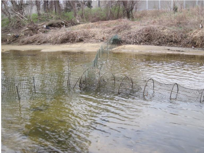
Figure 2. Block net (hoop net with deer fencing attached to block the creek) deployed in Cameron Run. The hedging is angled downstream in order to funnel up-migrating herring into the opening of the net.
